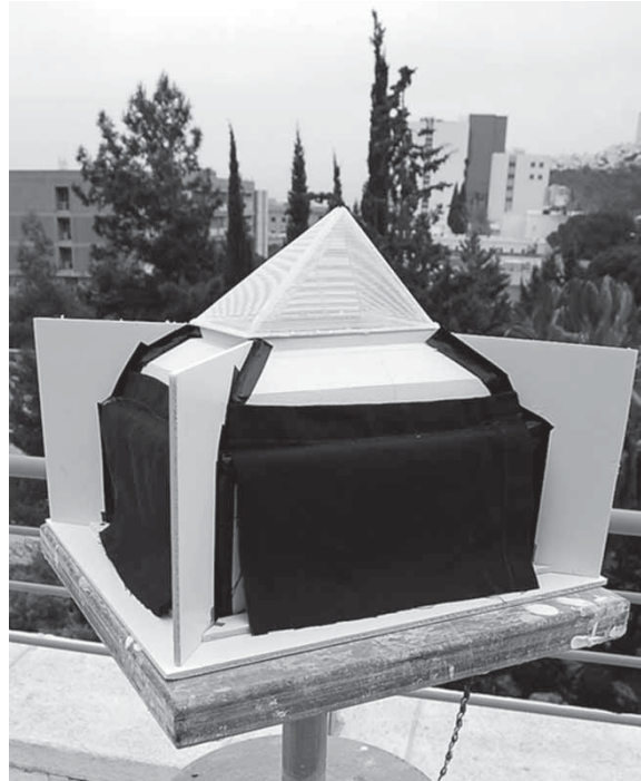
Figure 13. A 1:30 scale model of exhibition space and the proposed LCP gable.
